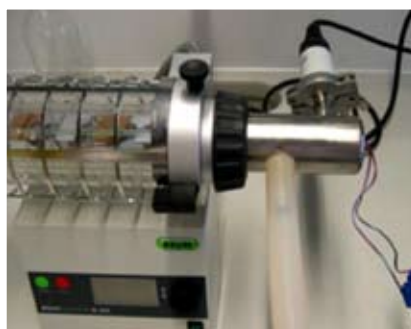
Fig 3: Customized extension of the drying chamber providing process control of product temperature and chamber pressure
