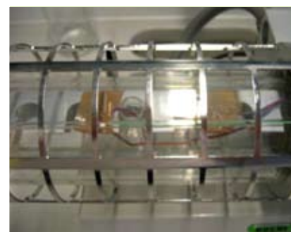
Fig 4: Placement of the two thermocouples monitoring the product temperature and glass wall temperature in the Glass Oven B-585
