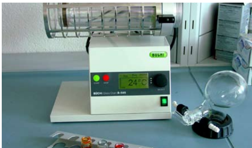
Fig 1: Glass Oven B-585 from Büchi Labortechnik AG with freeze drying option
