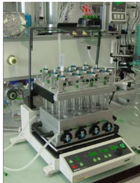
Figure 2: Syncore® Analyst with rack 12 and vacuum cover with SPE-cartridges
